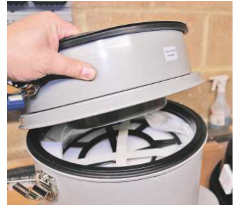
▲ The additional Hepa filter is optional to gain M class filtration levels
